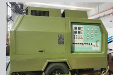
Mechanical equipment Air compressor contour noise equipment lined with sound-absorbing material
